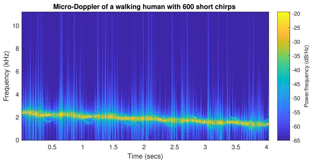
Figure 4.13: The spectrogram of a walking human with high resolution radar settings S1 .
