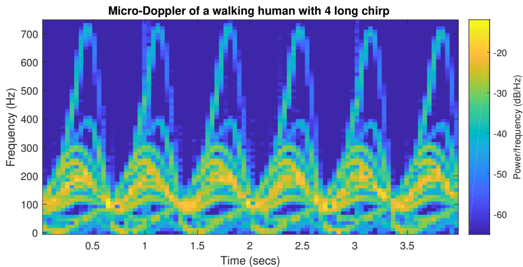
Figure 4.13: The spectrogram of a walking human with high resolution radar settings S1 .
