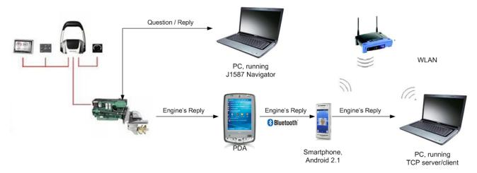
Figure 6.3: Hardware setup used for testing the PDA application
