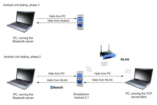
Figure 6.1: Hardware setup used for testing the Bluetooth and TCP server/client functionality on the smartphone
