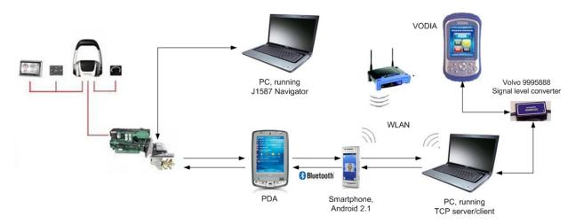
Figure 6.5: Hardware setup used for prototype's testing
