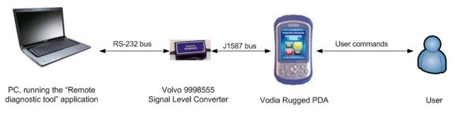
Figure 6.4: Hardware setup used for testing the "Remote diagnostic tool" – desktop application
