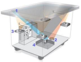
Figure 4. The inner parts of a Surface. 1: The screen. 2: Infrared lamp. 3: One of the infrared cameras. 4: Projector.
