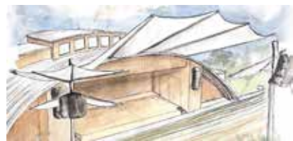
A protruding roof combats glare and rain, protecting the musicians and their instruments. It also covers part of the seated audience, helps guide music towards the lawn and connects the volumes.
