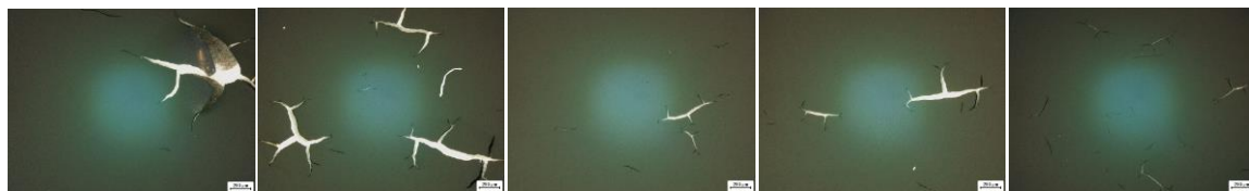
Figure 4.22: Microscope images for coatings at 150-micron coating height, left to right – dried at room temperature, 40 °C, 60 °C, 80 °C and 100 °C respectively.
