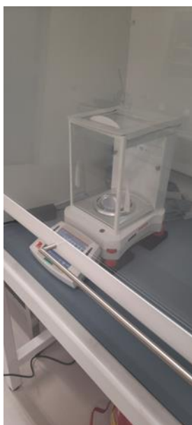
Figure 3.1: Weighing balance to measure and mix ink components to proportion.
