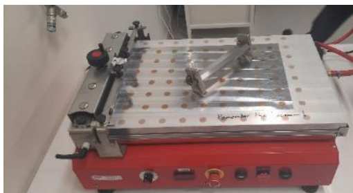
Figure 3.5: Doktor blade on the linear drive stage with a vacuum base
