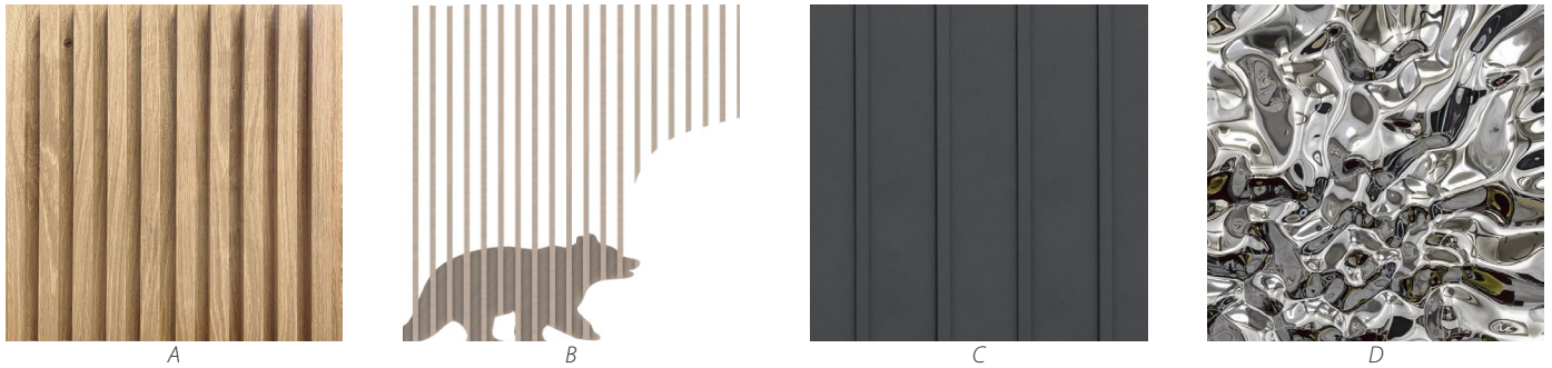
Figure 40. The facade is clad in unpainted wood (A), with 50 mm wide and 22 mm deep batten boards covering the backboards. In some places this pattern is disturbed by the storytelling facade pattern. In other places, it is up and aligns with the raster wood railing in the stairs (B) and on the northern balcony. The roof is dark metal (C), subtly hiding solar panels if those were to be installed. Where the facade meets the ground, a reflective metal sheet protects the wood from splashes and water damage. This metal is rippled in certain places, imitating water (D).
