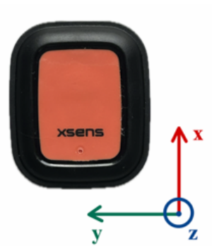
Figure 3.2: Local coordinate system of the Xsens IMU sensor.
