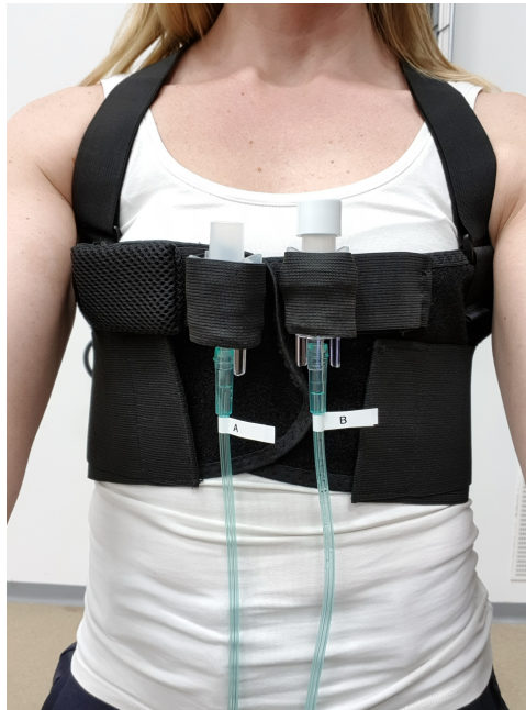
Figure 2.1: The fragrance administration system which was attached to a vest. The two tubes contained the two fragrances (A and B).
