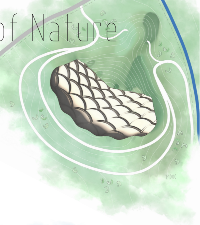
The grid shell is designed to act as a diffuser. The diffusive ceiling creates soft reflections, more even distribution in low domain and reduced echo. Different sizes of grid elements and distances between them provides effective diffusion in wide frequency range.
