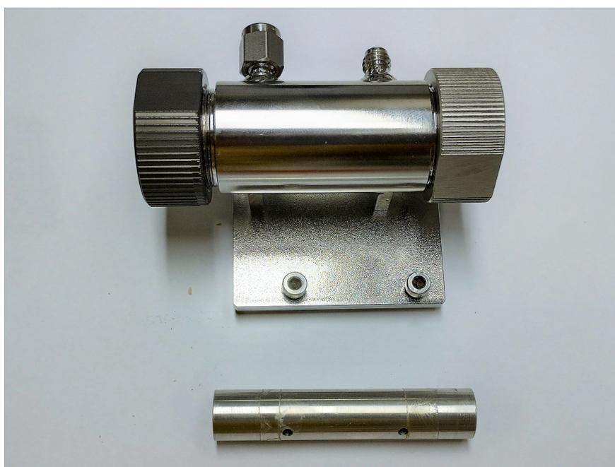
**Figure 4:** Modifications made to the FTIR gas cell
