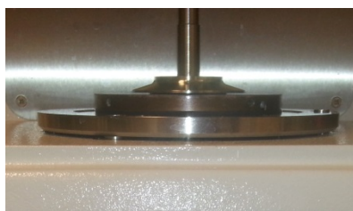
Figure 8. Sample solution put on plasma coated bottom plate. The different rheological information was accessed while applying different stress, frequency and temperature (Physica MCR 300 rheometer)
