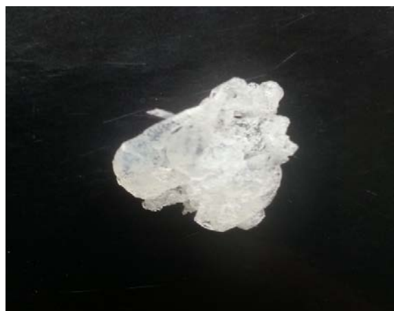
Figure 21. Dried coagulated sample ZnCl 2 :H 2 O (1:4, 40 °C, 600 rpm)
