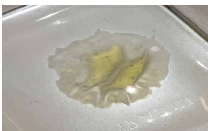
Figure 24. Coagulated cellulose obtained from the \text{ZnI}_2:\text{H}_2\text{O} molten salt
