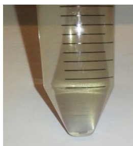
Figure 48. ZnCl 2 :H 2 O Fresh sample; Condition (1:4, 30 °C, 600 rpm)
