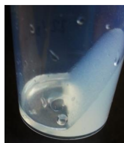
Figure 47. ZnCl 2 :H 2 O 7 days aged sample; Condition (1:4, 30 °C, 600 rpm)
