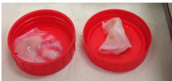
Figure 25. Wet coagulated samples ZnI 2 :H 2 O (1:5, 60 °C, 600 rpm)
