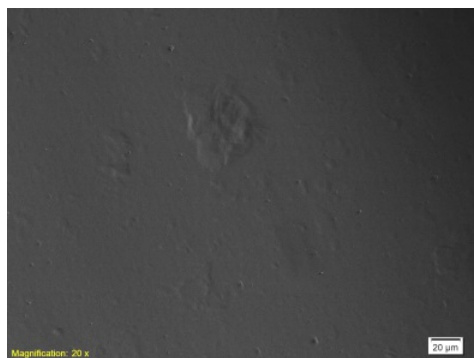
Figure 59. \text{ZnI}_2:\text{H}_2\text{O} (Aged >20 days) Light microscopy image, (1:5, 60 °C, 600 rpm)
