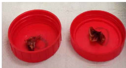
Figure 26. Air dried coagulated samples ZnI 2 :H 2 O (1:5, 60 °C, 600 rpm)
