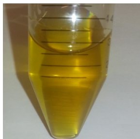
Figure 23. \text{ZnI}_2:\text{H}_2\text{O} (1:5, 60 °C, 600 rpm)
