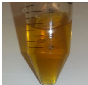
Figure 22. \text{ZnI}_2:\text{H}_2\text{O} (1:6, 60 °C, 600 rpm)
