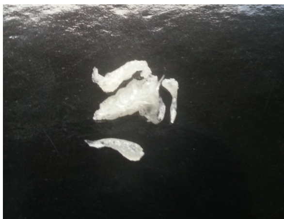
Figure 20. Dried coagulated sample ZnCl 2 :H 2 O (1:4, 40 °C, 400 rpm)
