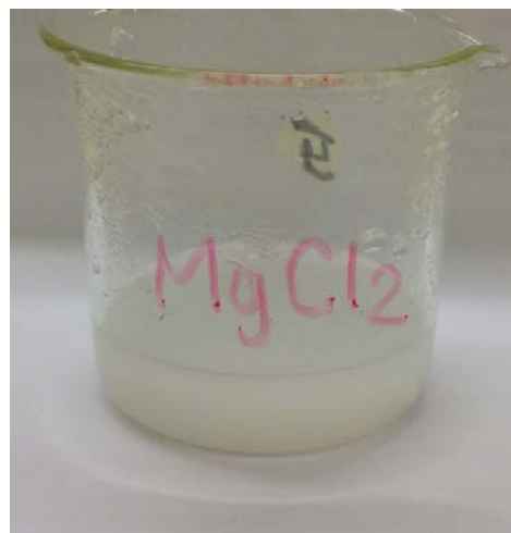
Figure 28. \text{MgCl}_2:\text{H}_2\text{O} (1:10, 60 °C, 600 rpm)
