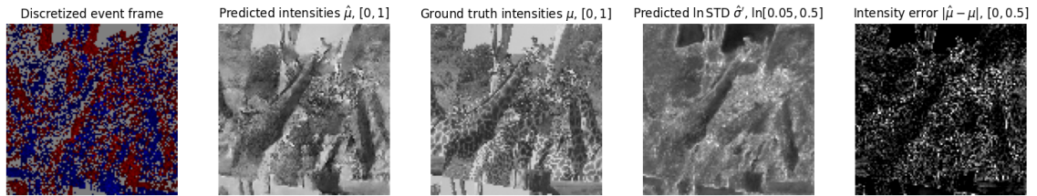
(a) LPIPS (Alex) = 0.292. With too many events, the method fails to reconstruct fine details, such as the giraffe coat patterns.
