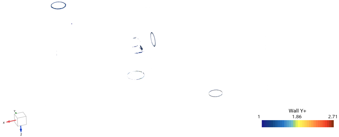
Figure 4.14: Wall Y^+ values of the reference simulation. Only wall Y^+ values above 1 are shown in the figure.
