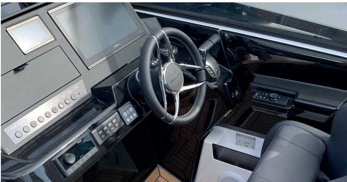
Figure 1: A cluttered helm station featuring a wide range of different components from different manufacturers.
