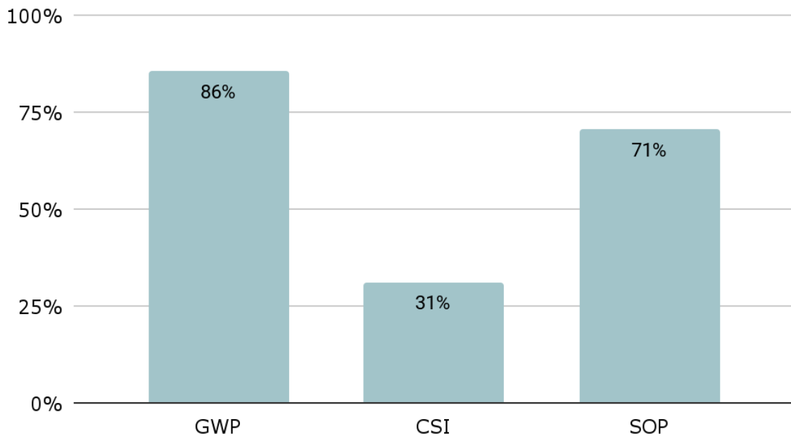
Figure 6.4: Effects on climate change and mineral resource depletion impacts when replacing silver (Ag) with magnesium (Mg).
