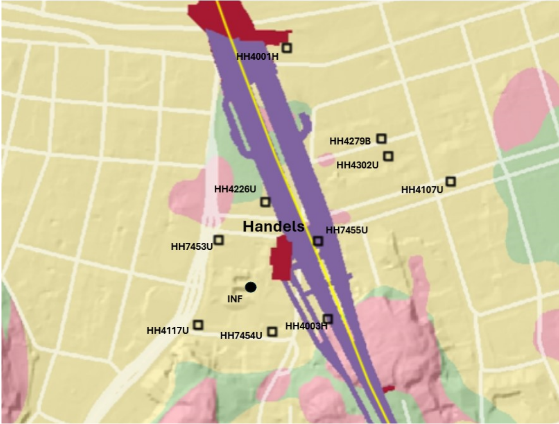
Figure 2.4: Map of the location of the wells. The Handels shaft is in the center with faint marking of fictional shafts and the tunnel. Wells, infiltration well (INF) and the Handels shaft are labeled.
