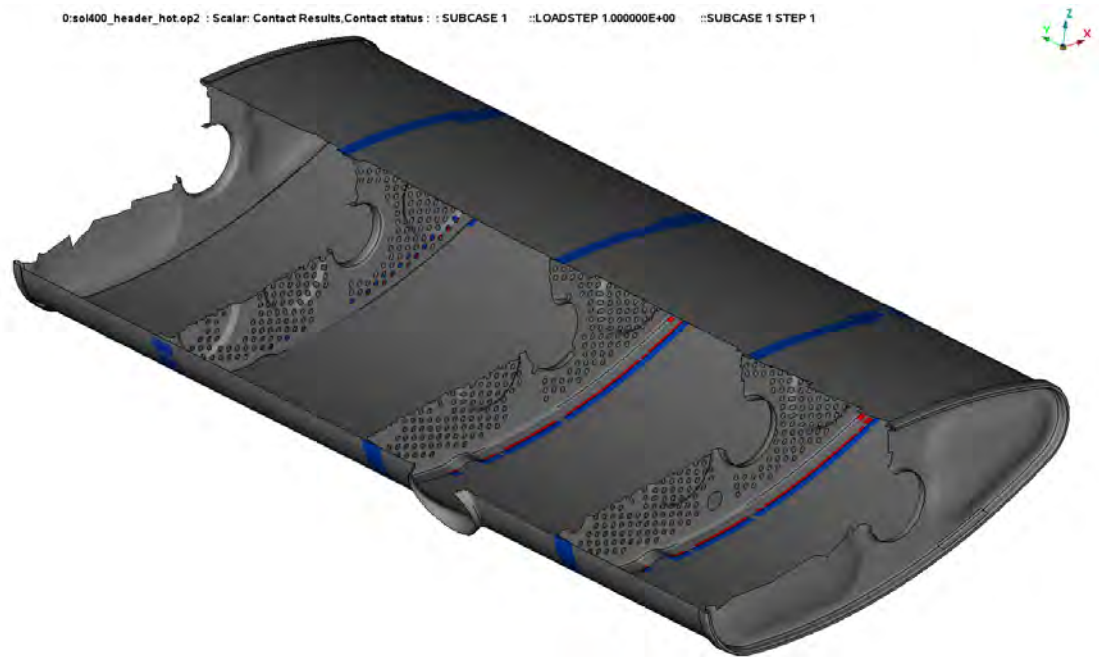
Figure 5.6.: Contact region identified by Sol 400.
