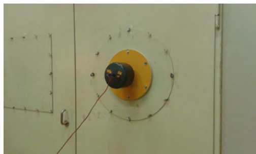
(g) Loudspeaker mounted on a door.
