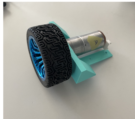
Figure 4.15: Motor and wheel mounted on bracket
