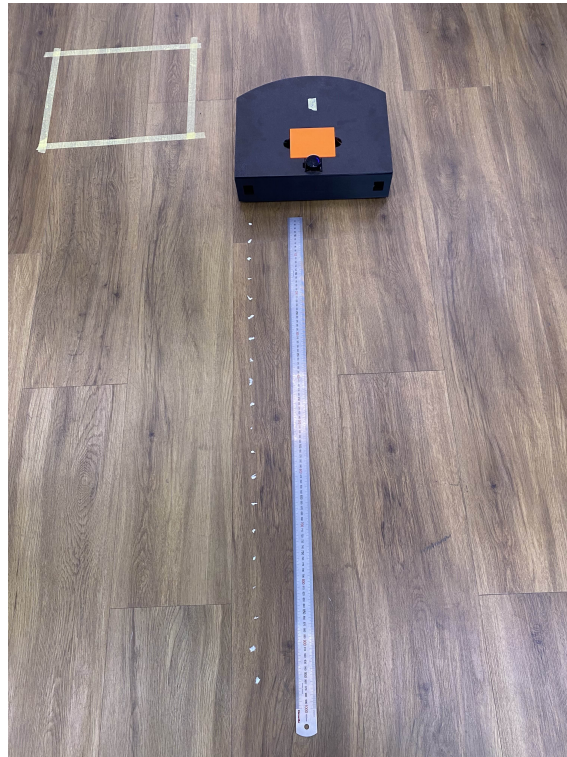
Figure 5.2: Brush performance test
