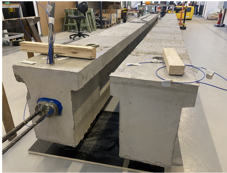
Figure 4.6: Specimens after casting and demoulding.
