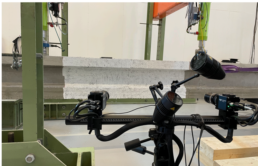
Figure 4.13: Setup for DIC and stochastic pattern on the specimen.
