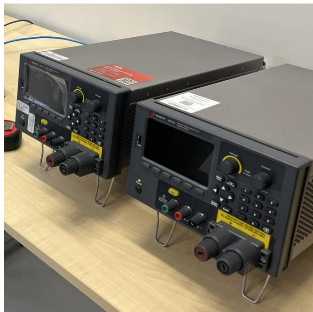
Figure 3.8: Two Keysight E36731A battery emulator and profiler.
