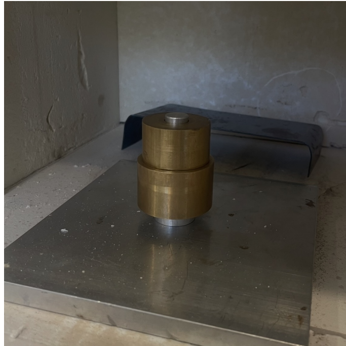
Figure 3.10: Test setup curing in the oven.
