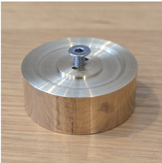
(a) Rigid mounting solution for \mathcal{A}_{i,j} .
