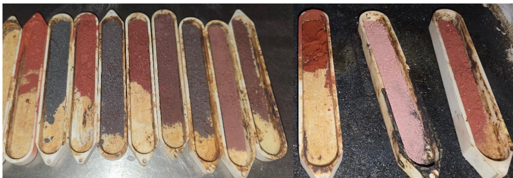
Figure 5: The samples 2 to 13, from left to right, containing the mixture after the addition of the PVA binder.
