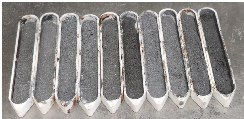
Figure 4: The samples 1.1 to 1.10, from left to right, containing the mixture after the addition of the PVA binder.
