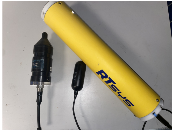
Figure 3.2: Example of the used hydrophones, left SoundTrap and right RTsys.
