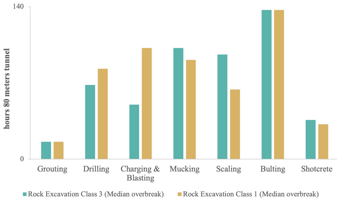
Figure 5.11: Time distribution in hours, for performing rock excavation with each rock excavation class, with median overbreak, for 80 meters tunnel in acceptable rock quality.
