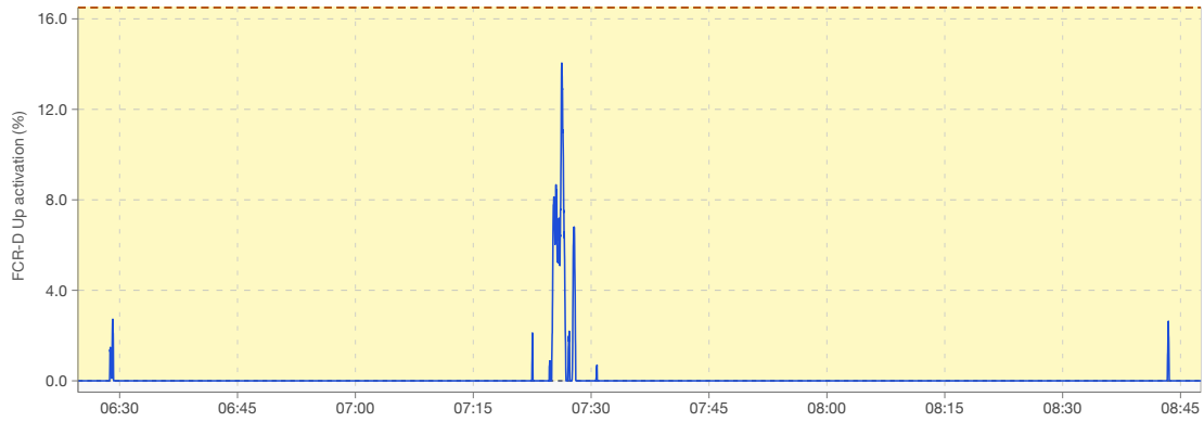
Figure 5.9: FCR-D Up activation on 2026-02-09 as a percentage of rated power derived from the frequency, shown over the morning interval that contains its events. Frequency data from [28].
