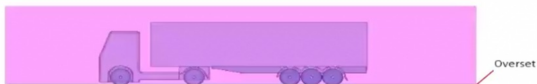
Figure 3.16: Representation of overset region around the truck
