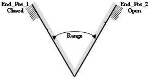
Figure D.3: Definition of actuator direction
