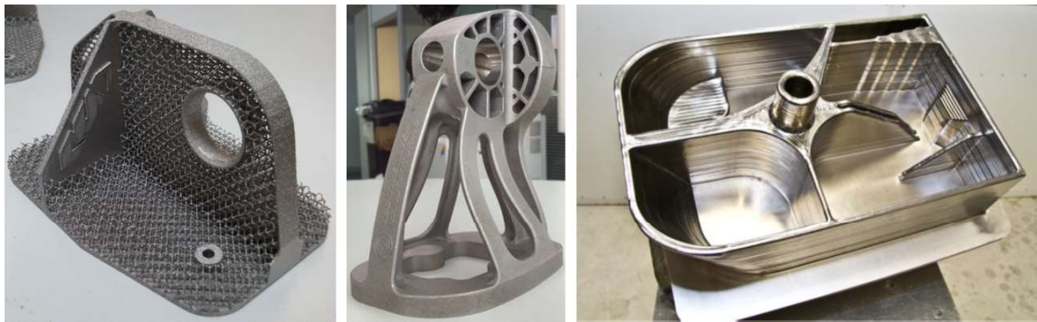
Figure 14: The two left components is made by PBF and the right by DED.
