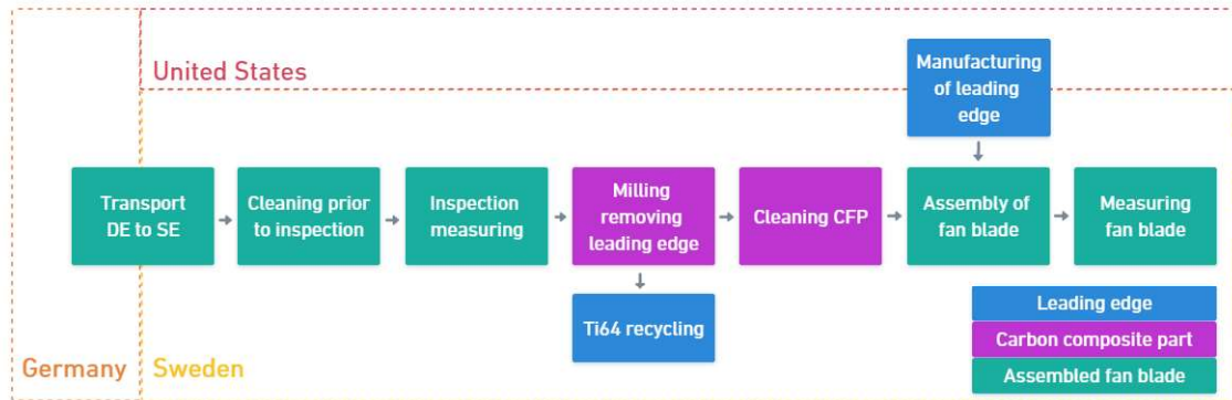
Figure 24: Flowchart illustrating the processes of CM repair.
