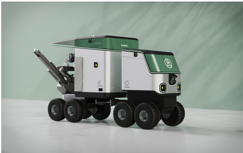
Figure 1.1: The BraSatt prototype BraSatt 01 shown in a rendered picture. The vehicle is approximately 4 m long and 2.4 m high.
