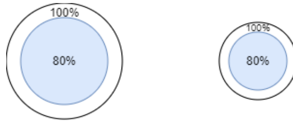
Figure 2.13: Visualizing the difference between an 80% open valve for a large pipe and an 80% open valve for a small pipe.
