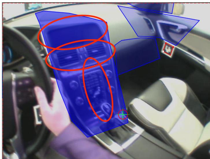
**Figure 30:** A potential AOI, the Center Stack, including smaller components such as the stereo, central air vents, and the central display (Print screen from D-lab 2.5).
