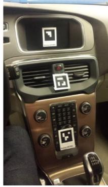
**Figure 18:** Example of attachment of markers on the Instrument Panel and center Display.
