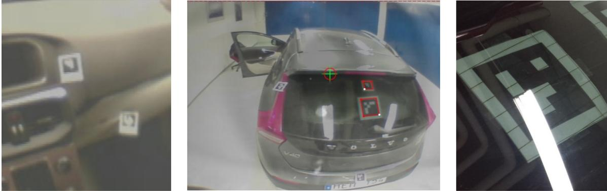
**Figure 23:** To the left, white area of markers has melt together. In the middle, the markers could be recognized when hidden under the car window. To the right, the marker is not detected due to a reflective light source in the glass.
