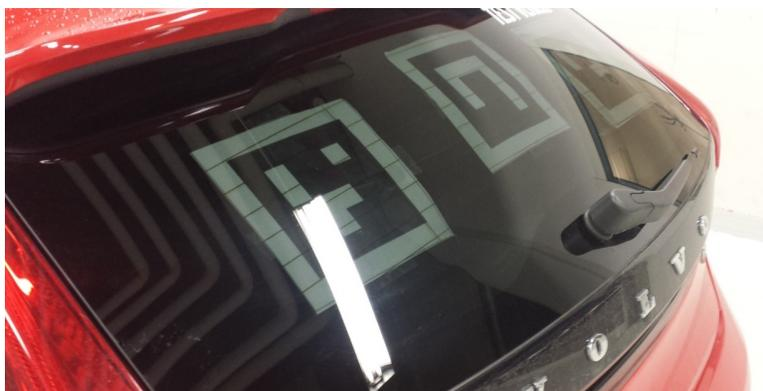
**Figure 28:** Picture showing how one marker is still visible when one is covered by a reflecting light source.
