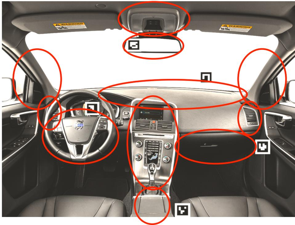
**Figure 34:** The final suggestion on which AOI's to use and how to place the markers in the Main Study.
