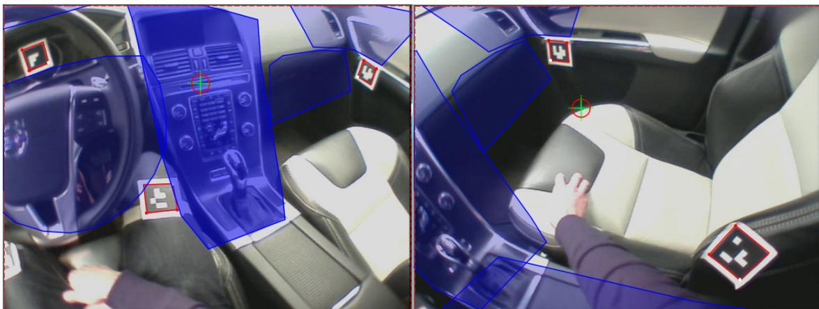
**Figure 29:** To the left, AOI drawn while direct staring at the center stack. To the right, instability of the center stack as the AOI has been drawn at the wrong moment (Print screen from D-lab 2.5).
