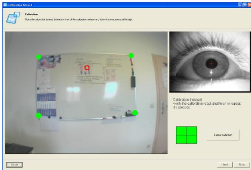
**Figure 12:** All four calibration points displayed with green markers (Ergoneers.Group, 2011).
