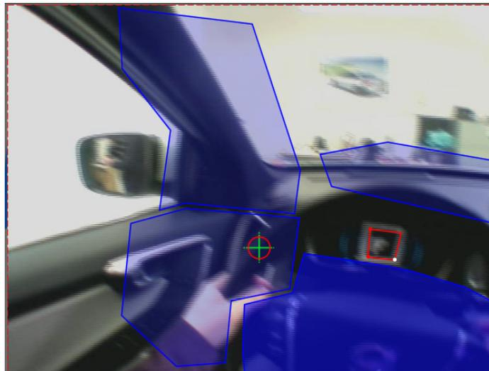
**Figure 44:** Showing AOI’s closely placed which may result in “near” correlation (Print screen from D-lab 2.5).
