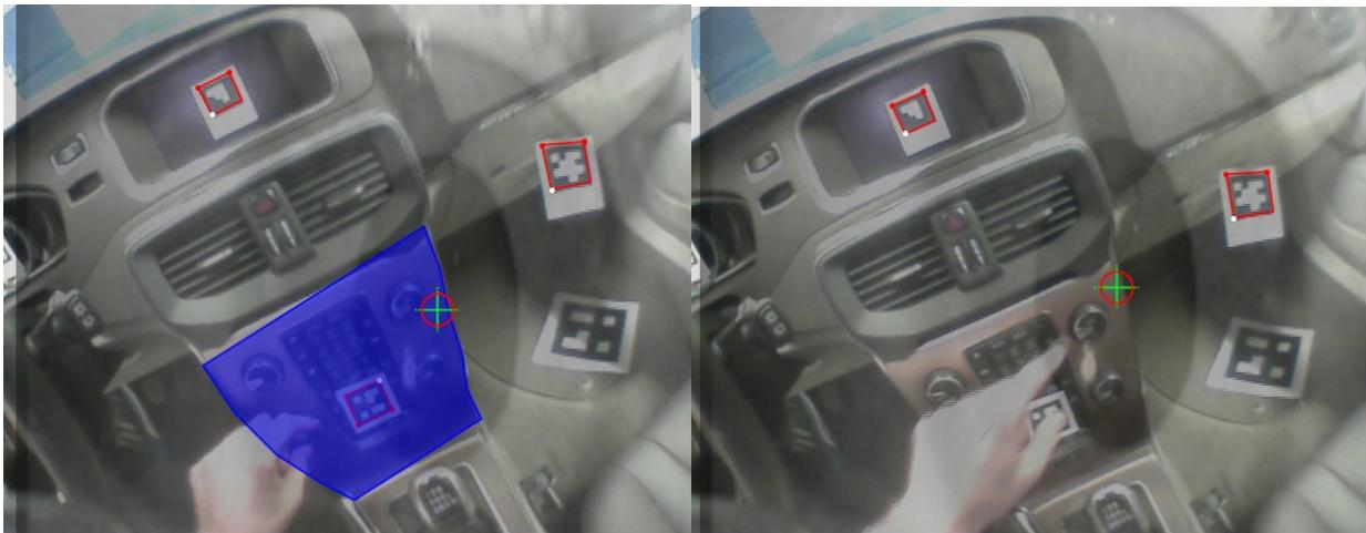
**Figure 22:** To the left, the marker connected to the AOI of the IP was visual. To the right, the marker was covered while using the buttons on the IP and the AOI was lost (Print screen from D-lab 2.5).
