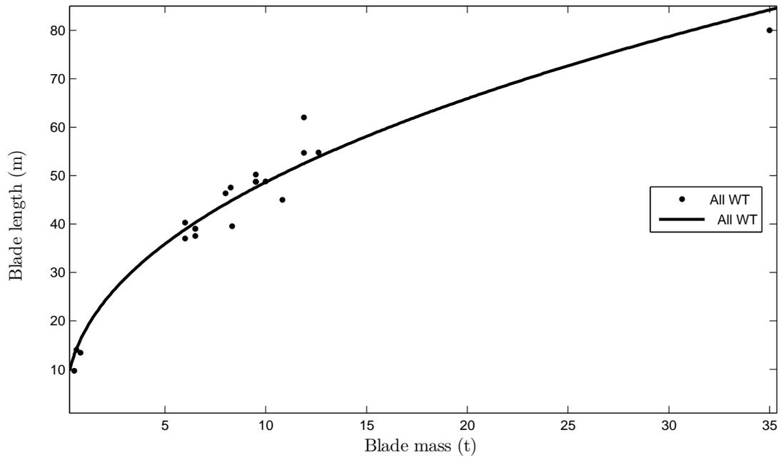
Figure B.7: *Evolution of the blade mass with respect of the blade length*
