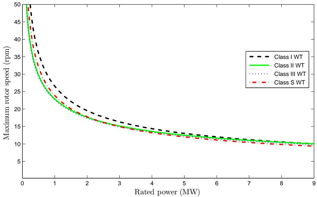
Figure B.6: Evolution of the maximum rotor speed with respect of the rated power: different WT classes
