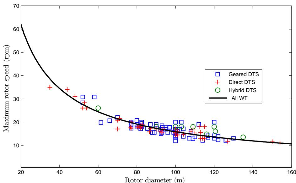
Figure 3.18: *Evolution of the maximum rotor speed with respect of the diameter: All WTs*
