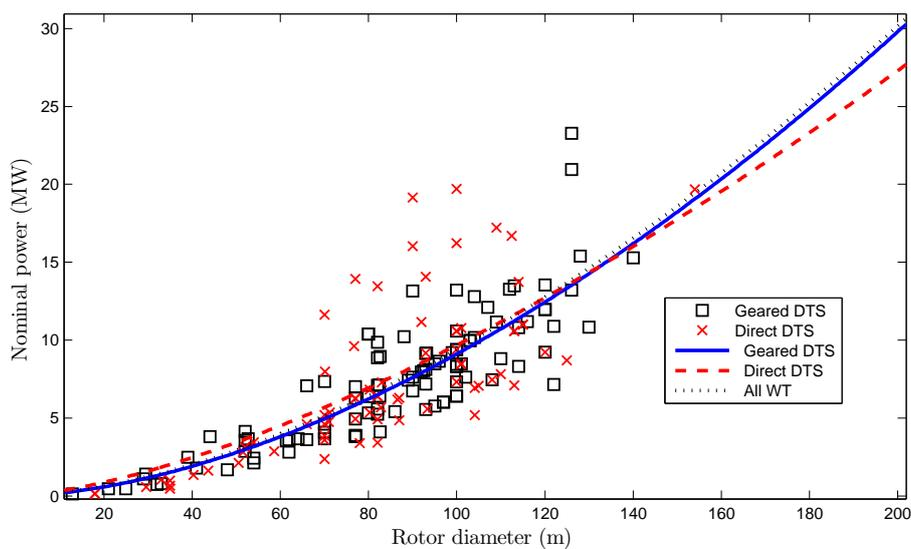
Figure 3.26: *Evolution of the Nominal power with respect of the rotor diameter: different DTS*
