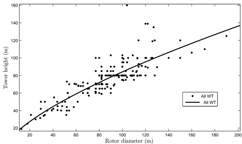
Figure 3.9: *Evolution of the tower height with respect of the rotor diameter*
