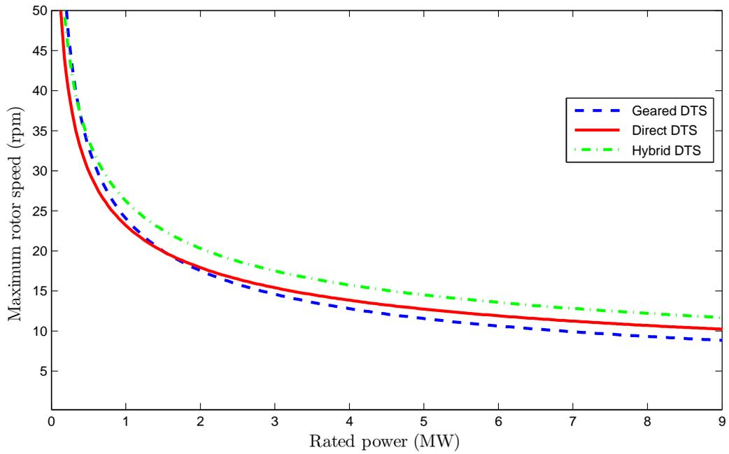
Figure B.5: Evolution of the maximum rotor speed with respect of the rated power: different DTS
