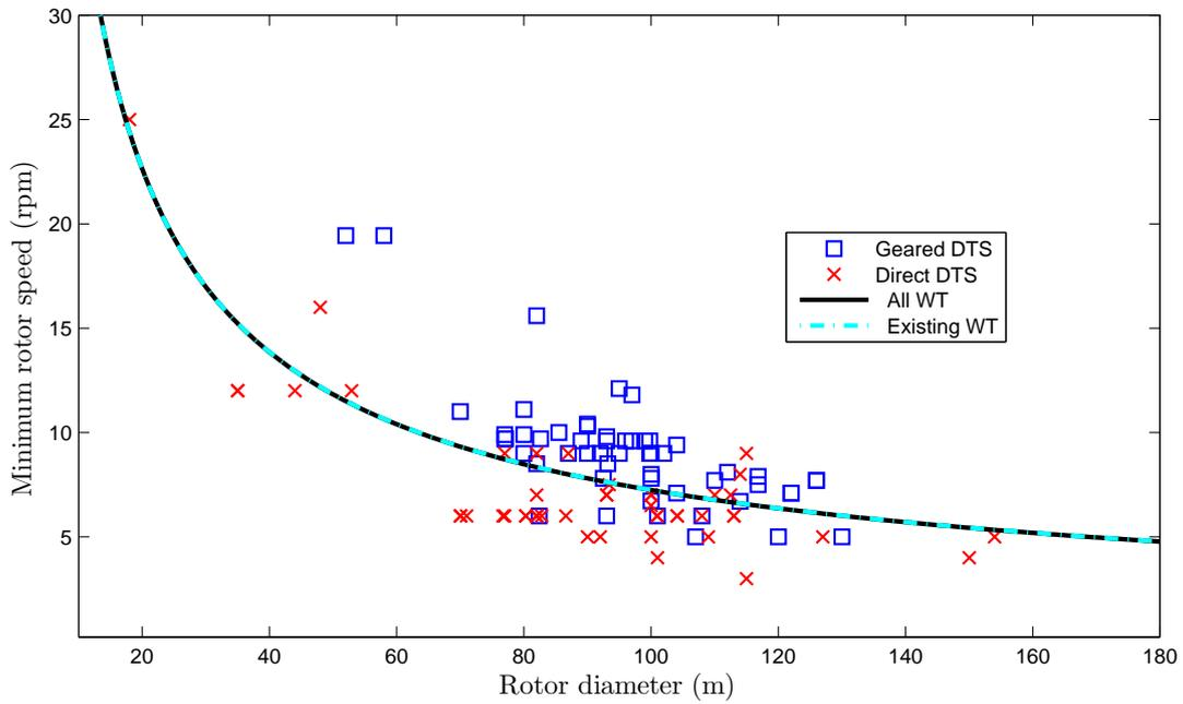
Figure B.2: Evolution of the minimal rotor speed with respect of the rotor diameter: All WT
