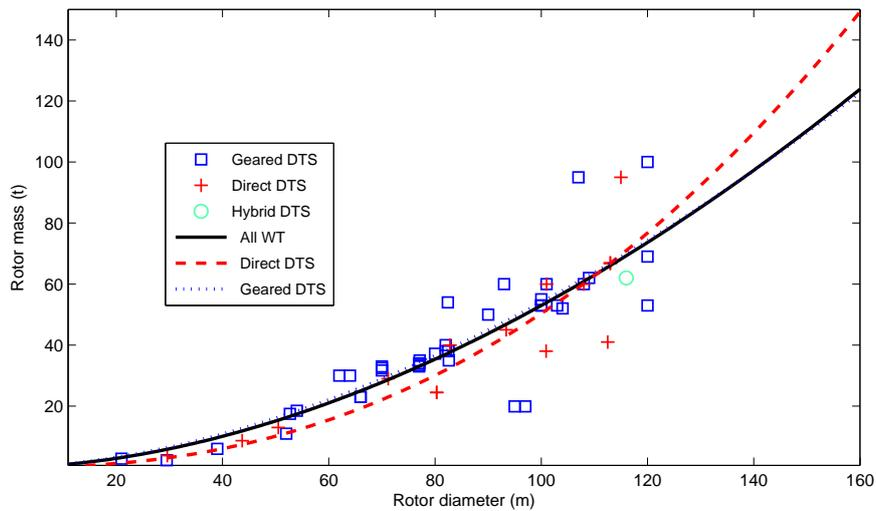
Figure 3.12: *Evolution of the rotor mass with respect of the rotor diameter*
