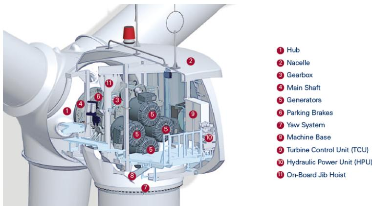
Figure 2.6: *Hybrid DTS with multiple generators [12]*
