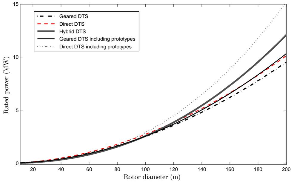
Figure 3.7: *Evolution of the rated power with respect of the rotor diameter: Different DTS*
