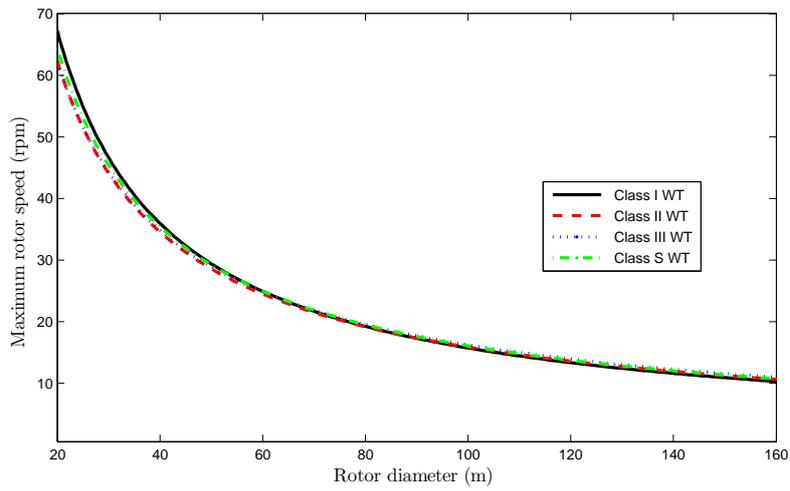
Figure 3.20: Evolution of the maximum rotor speed with respect of the diameter: WT classes
