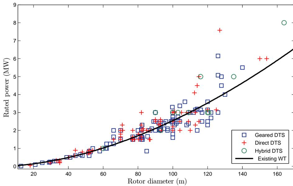
Figure 3.5: *Evolution of the rated power with respect of the rotor diameter: existing WT*
