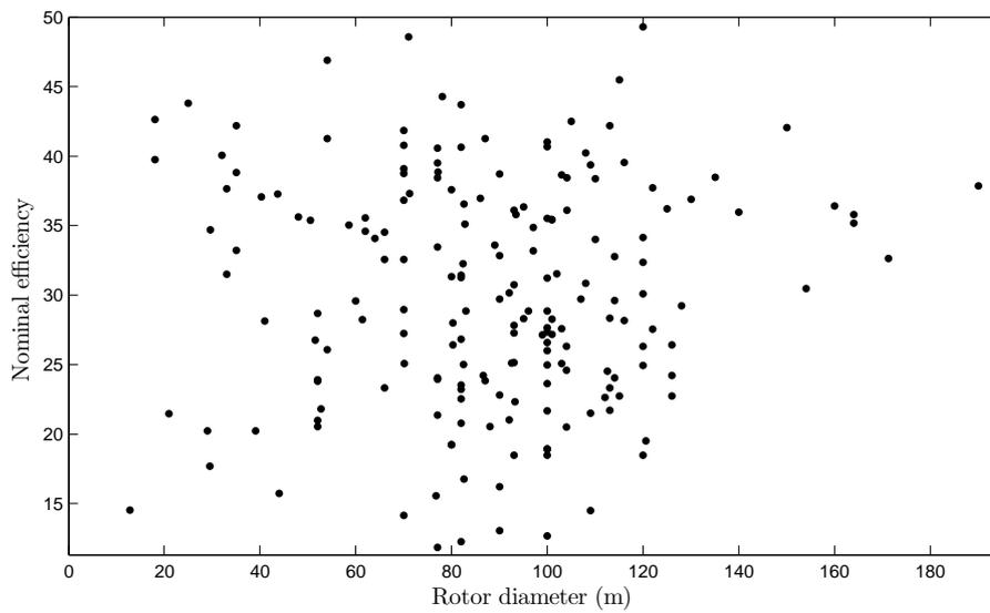
Figure 3.27: *Evolution of the Nominal efficiency with respect of the rotor diameter*
