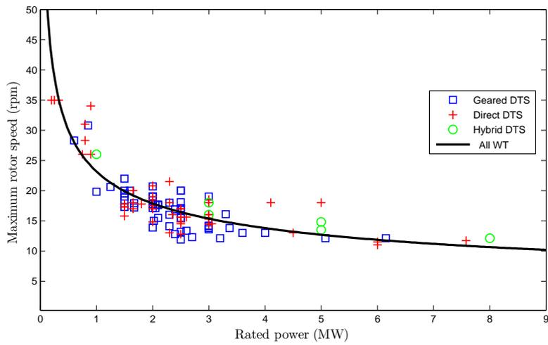
Figure 3.21: Evolution of the maximum rotor speed with respect of the rated power
