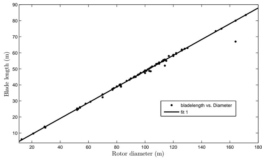
Figure 3.8: *Evolution of the blade length with respect of the rotor diameter*
