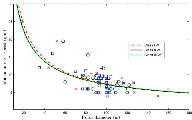
Figure 3.22: Evolution of the minimum rotor speed with respect of the diameter: WT classes
