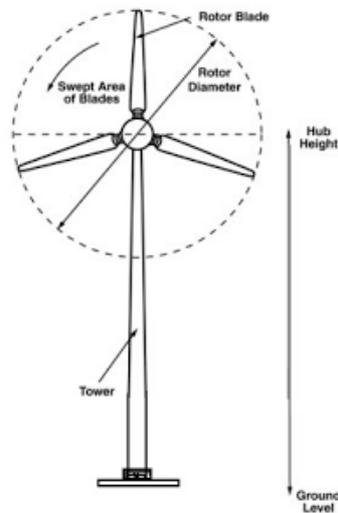
Figure 3.1: *Rotor diameter, swept area and hub height [17]*
