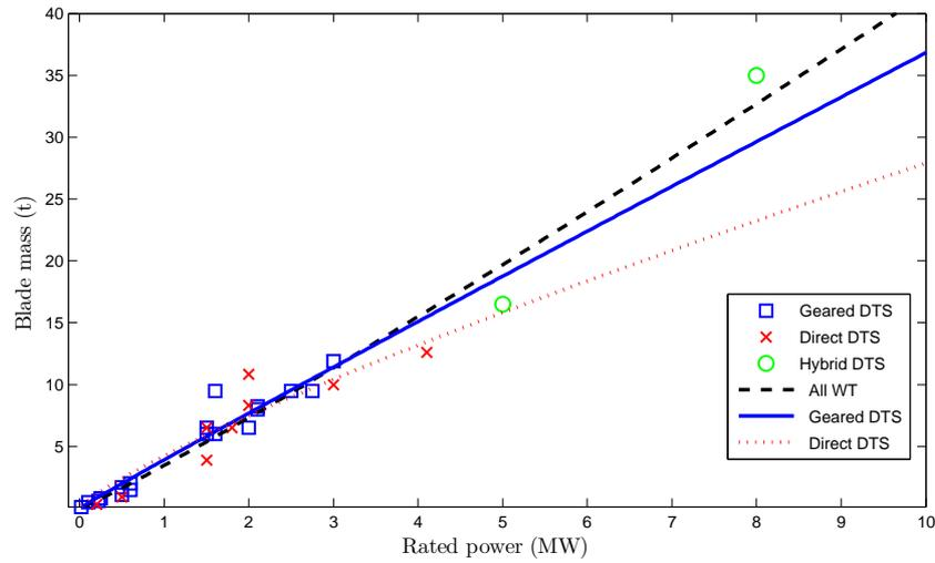
Figure 3.11: *Evolution of the blade mass with respect of the rated power: types of DTS*
