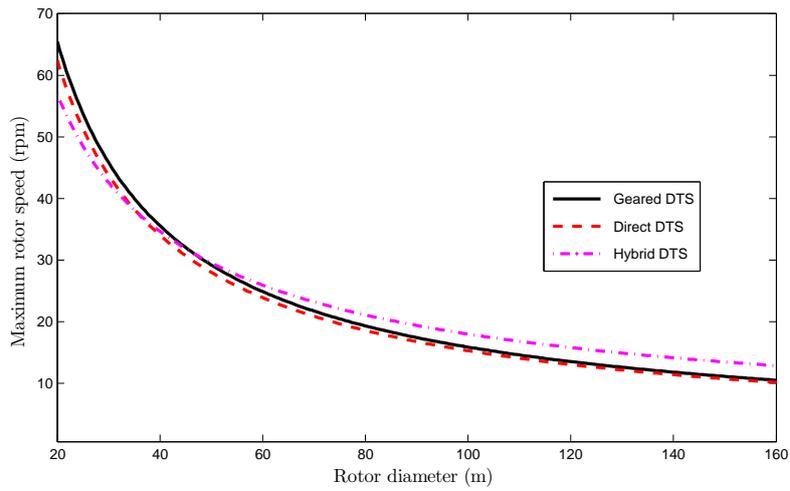
Figure 3.19: Evolution of the maximum rotor speed with respect of the diameter: types of DTS
