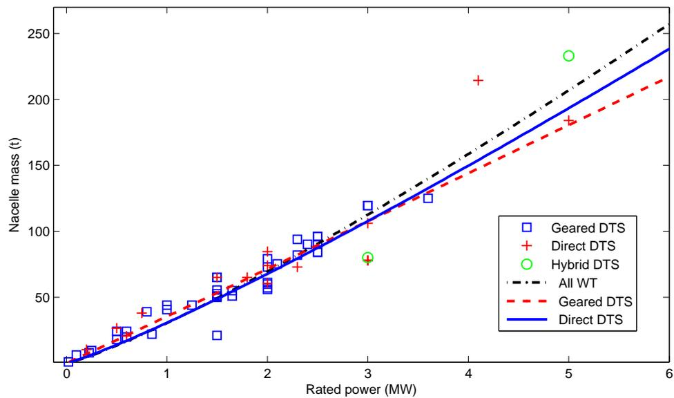
Figure B.3: Evolution of the nacelle mass with respect of the rated power
