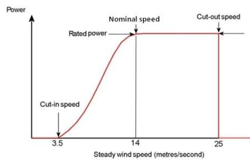
Figure 3.2: *Typical wind turbine power output with steady wind speed [18]*
