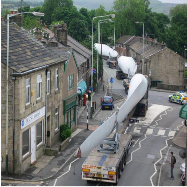
Figure 3.30: *Transport of a 48.5 m blade [25]*
