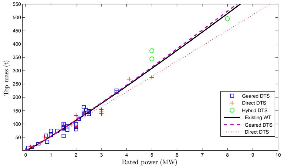
Figure 3.15: *Evolution of the Top mass with respect of the rated power*
