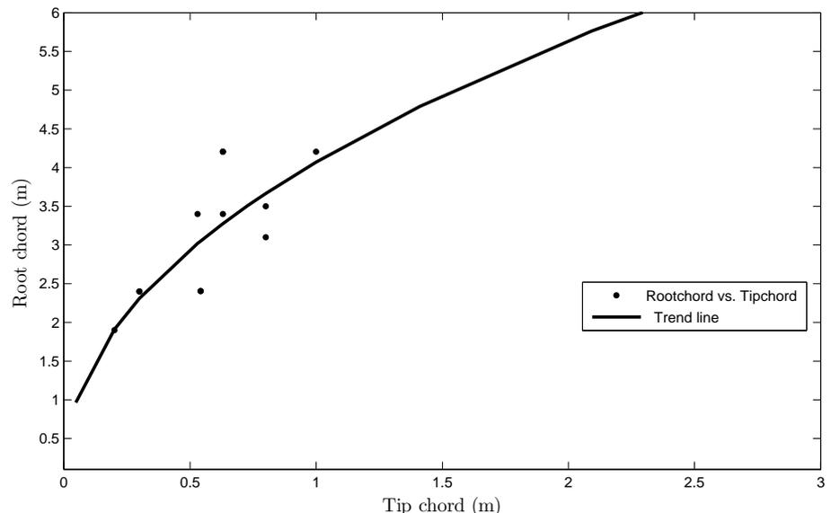
Figure 3.17: Evolution of the root chord with respect of the tip chord
