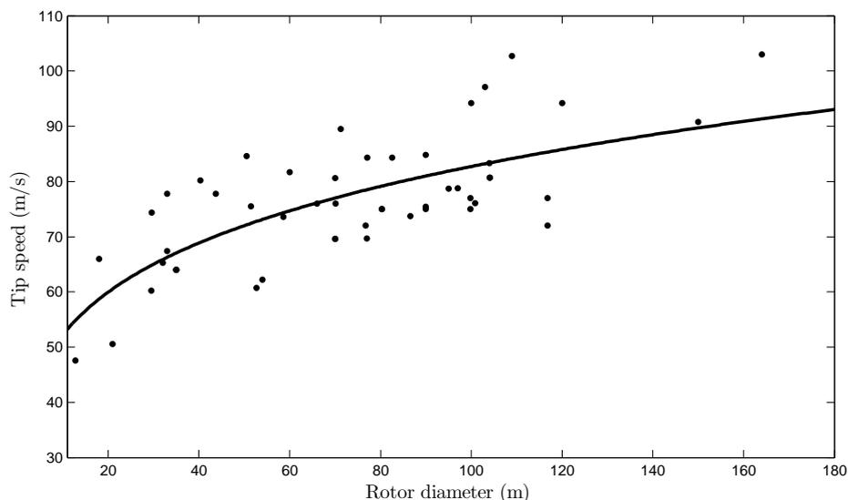
Figure 3.24: Evolution of the tip speed with respect of the rotor diameter
