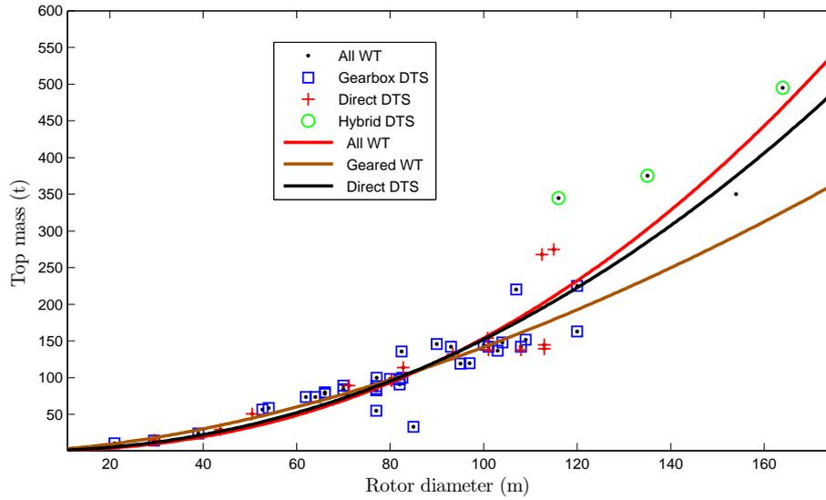
Figure 3.14: *Evolution of the Top mass with respect of the rotor diameter*
