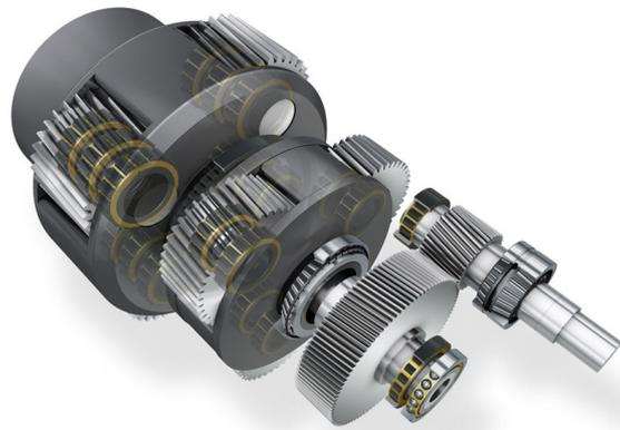
Figure 2.5: *Common gearbox in WTs [9]*
