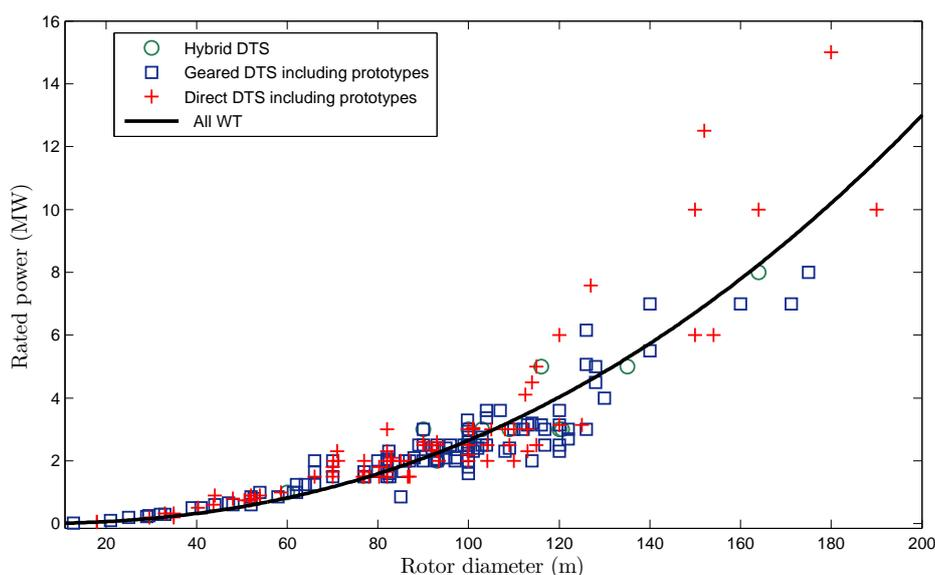
Figure 3.4: *Evolution of the rated power with respect of the rotor diameter: all WT*
