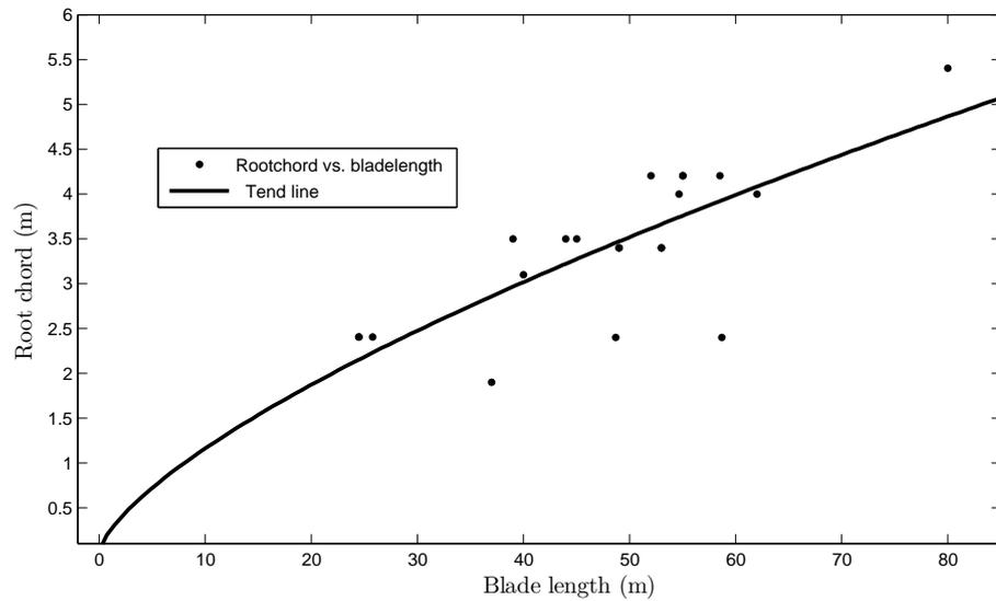
Figure 3.16: Evolution of the root chord with respect of the blade length
