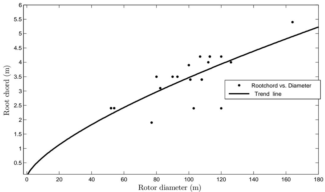
Figure B.1: *Evolution of the root chord with respect of the rotor diameter*
