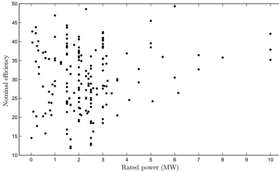
Figure 3.28: *Evolution of the Nominal efficiency with respect of the rated power*
