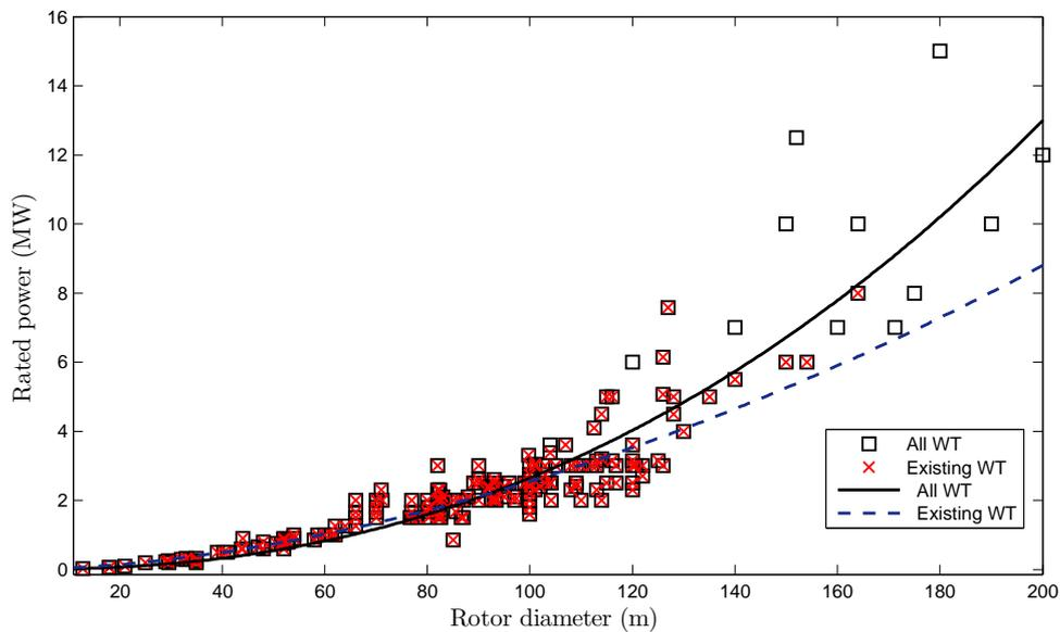
Figure 3.6: *Evolution of the rated power with respect of the rotor diameter: real and prototypes WTs*
