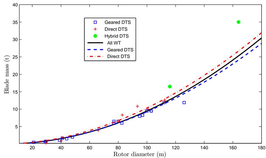
Figure 3.10: *Evolution of the blade mass with respect of the rotor diameter*
