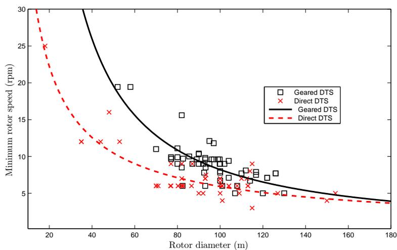
Figure 3.23: Evolution of the minimum rotor speed with respect of the diameter: types of DTS
