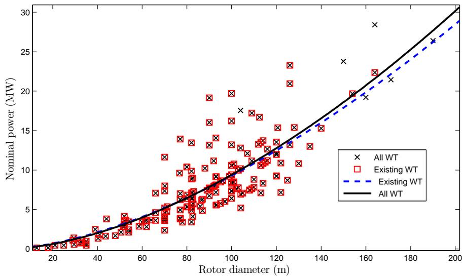
Figure 3.25: *Evolution of the Nominal power with respect of the rotor diameter*
