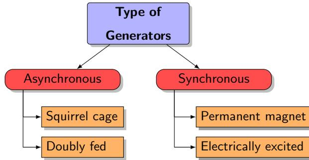
Figure 2.9: Main types of generators used in WTs
