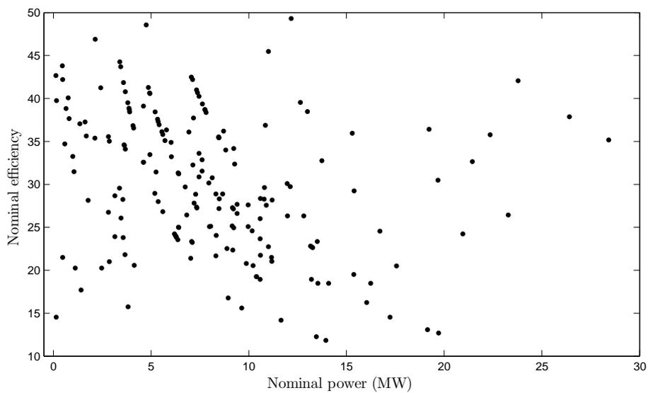
Figure 3.29: *Evolution of the Nominal efficiency with respect of the nominal power*
