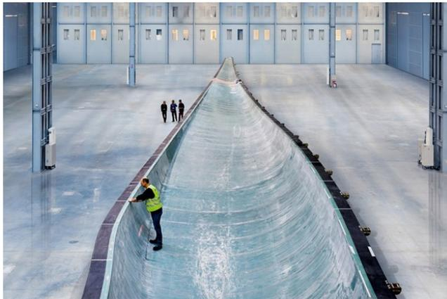
Figure 3.31: *Mould used to manufacture the 75m Siemens blade [26]*
