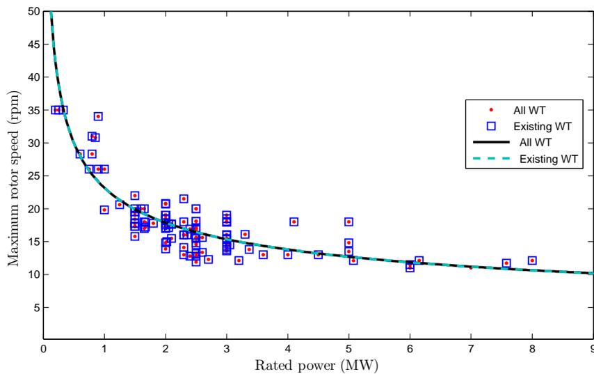
Figure B.4: Evolution of the maximum rotor speed with respect of the rated power: All WTs
