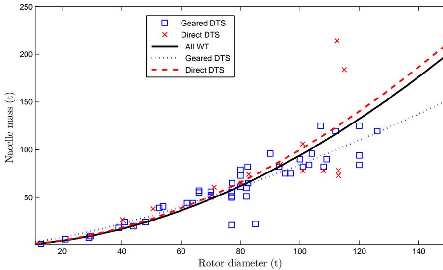
Figure 3.13: *Evolution of the Nacelle mass with respect of the rotor diameter*
