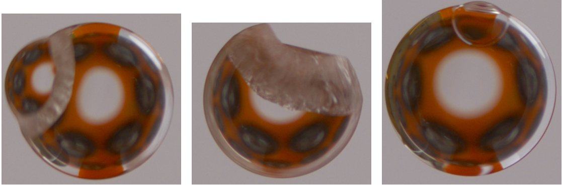
Figure 4.4: a) Water droplet of 1 \mu\text{L} (up left) and hexadecane droplet of 3 \mu\text{L} (right side) the moment after hexadecane was added. Here it is clear that the surface of hexadecane begins to freeze, b) water was almost completely evaporated and the bowl-like structure was formed, c) hexadecane melted and a low-volume water droplet still remained visible at the top of the hexadecane droplet.
