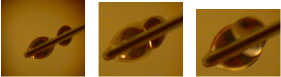
Figure 4.1: Sequence of three images captured at a time interval of 1/50 second, a) depicts hexadecane droplets suspended from a needle tip, with a neighboring water droplet, b) the hexadecane and water droplets are in close proximity, but have not made contact, yet, c) the moment when the hexadecane and water droplets came in contact. Notably, the onset of hexadecane freezing is evident.
