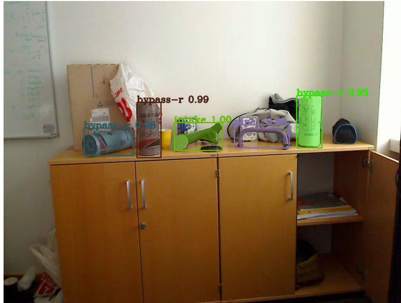
Figure 6.9: Inference on a real cluttered scene with the model trained without augmentations.
