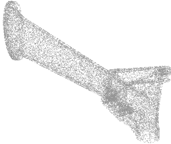
Figure 4.15: Properly sampled mesh of the intake with 20 000 samples.
