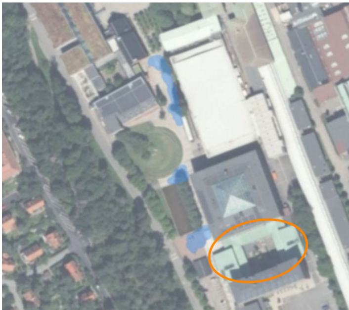
Figure 18. Overview of areas for stormwater problems on the site. Blue markings show visible floodings during normal rain and orange circles show where the significant copper sources (roofs) can be found in the area.
