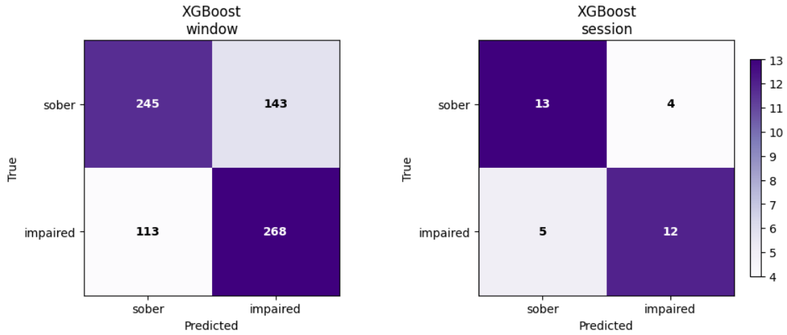
Figure 4.5: Confusion matrix for XGBoost trained on simulator data and tested on external real-world driving data at decision threshold 0.6.
