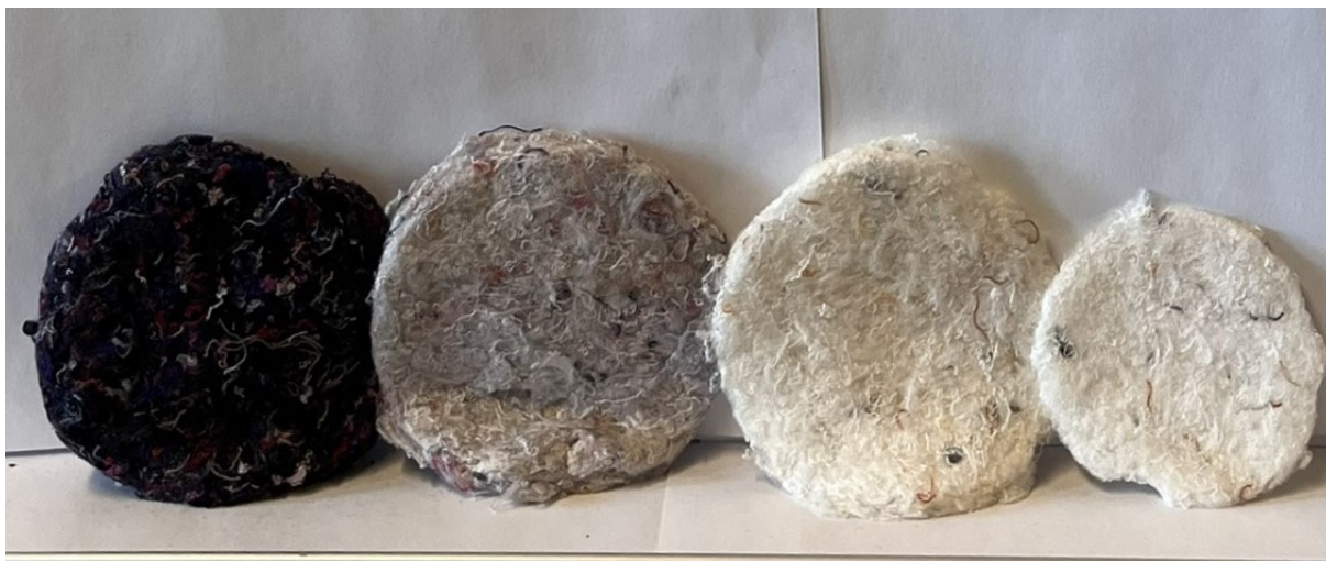
Figure 4.16: Viscose samples obtained by decolorizing with different stages and subsequences of EDP-sequence, from left to right: reference, E, ED and EDP. (Sheet size differ due to different amount of fibers, not due to yield losses.)
