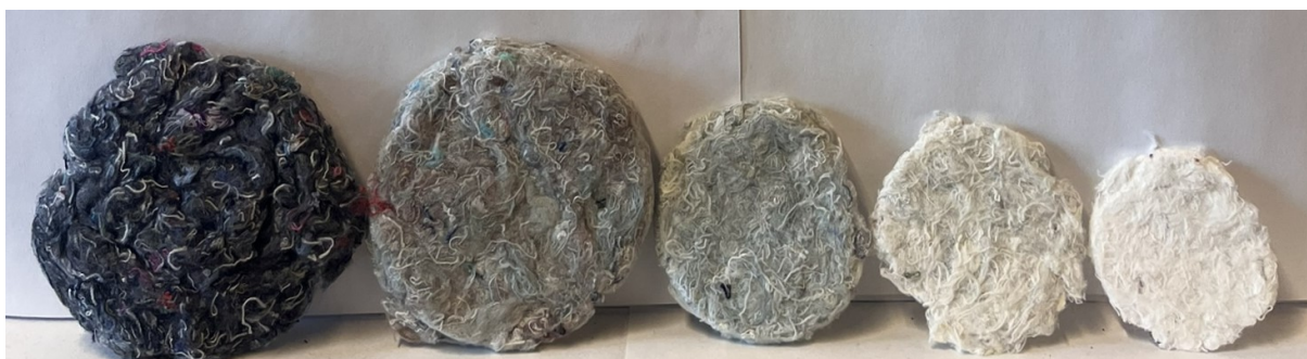
Figure 4.15: Cotton samples obtained by decolorizing with different stages and subsequences of EYDP-sequence, from left to right: reference, E, EY, EYD and EYDP. (Sheet size differ due to different amount of fibers, not due to yield losses.)
