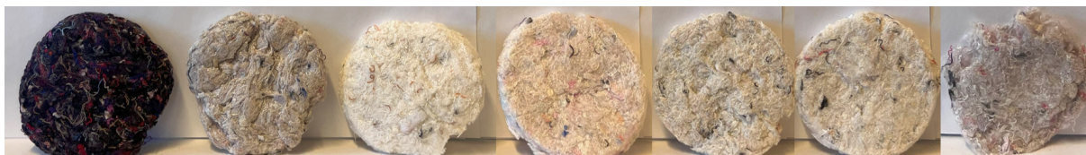
Figure 4.13: Double treated samples of viscose, from left to right: Reference, E, ED, EP(alk.), EP(Fenton), EZ and EY.
