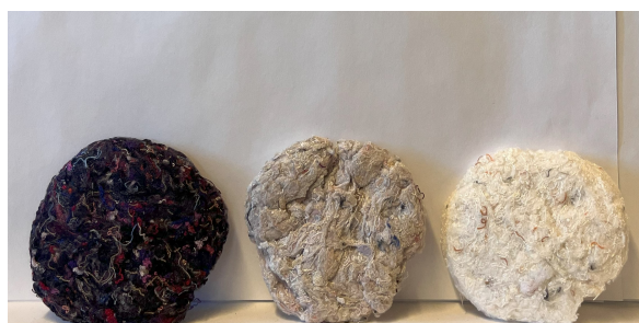
(c) Viscose samples from ED-treatment, from left to right: reference, E-treated, ED-treated.
