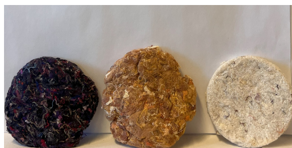
(d) Viscose samples from DE-treatment, from left to right: reference, D-treated, DE-treated.
