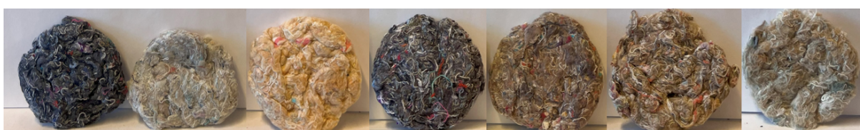
Figure 4.9: Single stage treated samples of cotton, from left to right: reference, E, D, P(alk.), P(Fenton), Z and Y.
