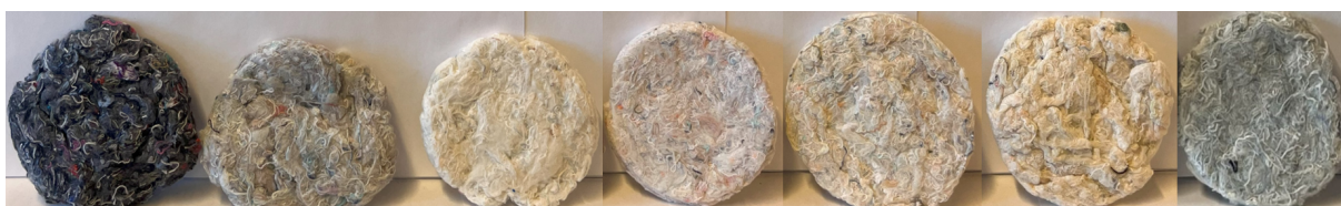
Figure 4.12: Double treated samples of cotton, from left to right: Reference, E, ED, EP(alk.), EP(Fenton), EZ and EY.
