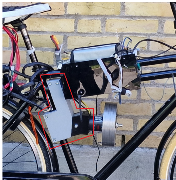
Figure 4.3: Finished Grey Actuator Mount
