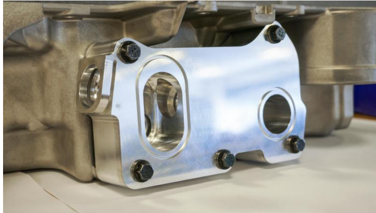
Figure 5.32: The prototype of the adapter plate fitted on the oil pan.
