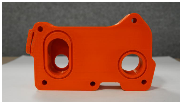
Figure 5.31: The 3D printed adapter plate.
