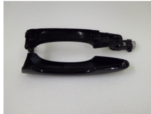
Fig. A.11.: Keyless handle, removed electrics, 70 g.
