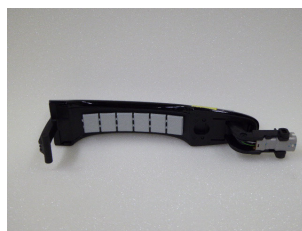
Fig. A.13.: Keyless handle with additional mass, 185 g.
