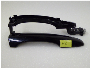
Fig. A.11.: Keyless handle, removed electrics, 70 g.
