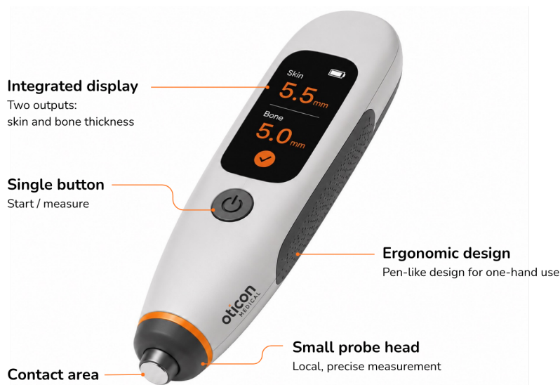
Figure 6.2: Conceptual visualization of a possible future handheld ultrasound device with an integrated display showing determined skin and bone thicknesses as output. Image generated using ChatGPT (OpenAI, 2026).
