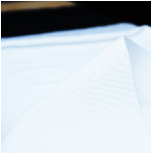
Textile - 100% polyester, woven at Swedish School of Fashion, coated with nano material fluorocarbon for water and dirt resistance
