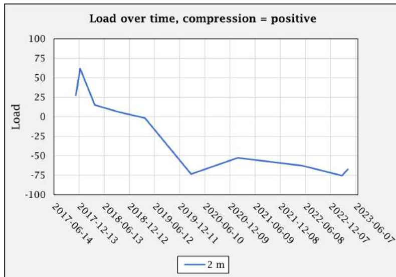
Figure E.0.1: Evaluated load 2 metres from the top of pile 3-417, located in the center wall.
