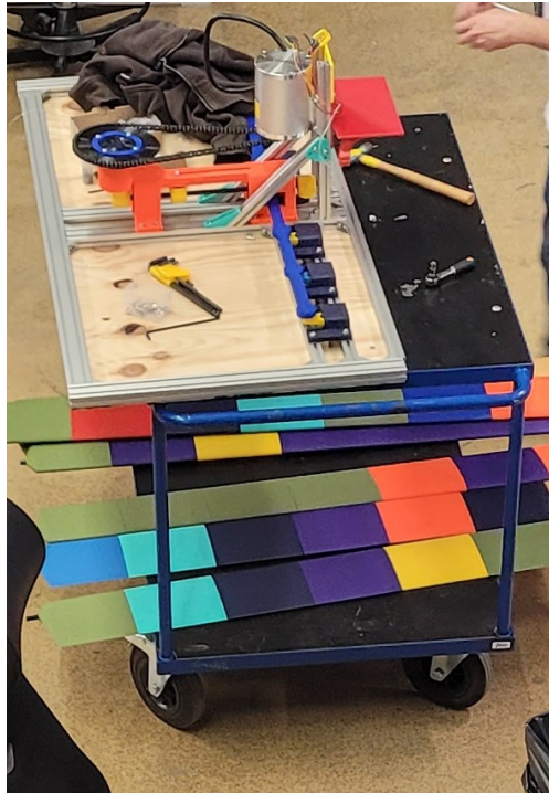
Figure 3.24: Aluminum profile with wooden plate
