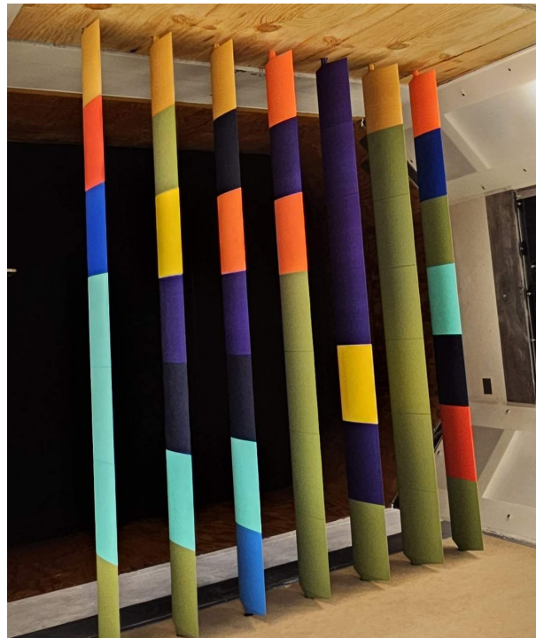
Figure 2.14: Active turbulence generator
