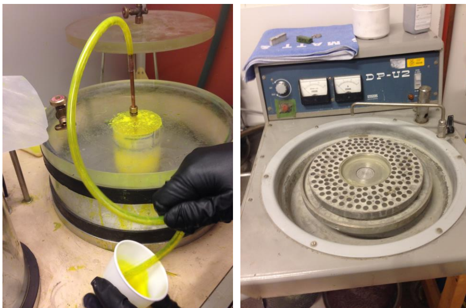
Figure 11: Left: Impregnation of epoxy resin. Right: Polishing device.
