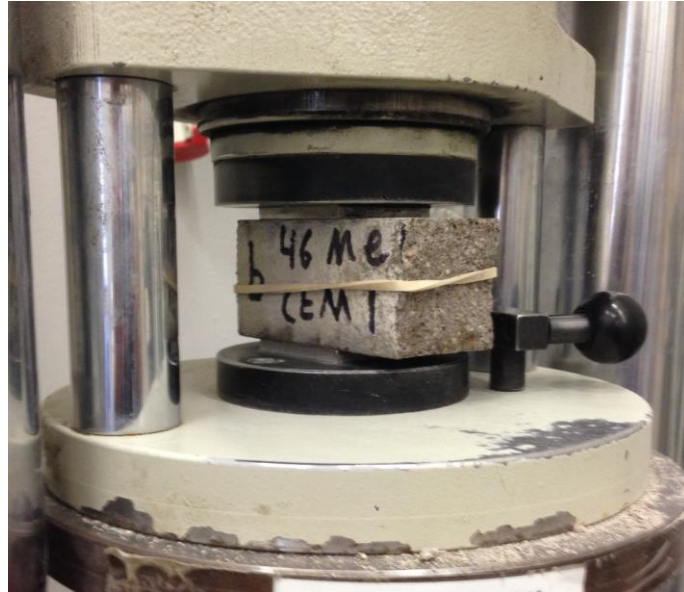
Figure 10: Testing of the compressive strength for one half of a prism.
