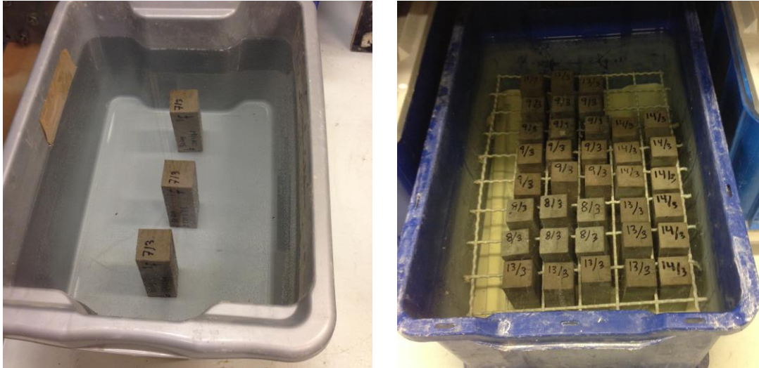
Figure 8: Left: One of the low pH storage containers. Right: The high pH storage container.
