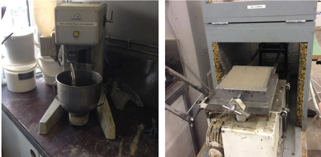
Figure 9: Left: Hobart mixer. Right: A mould filled with cement placed on the jolting table.
