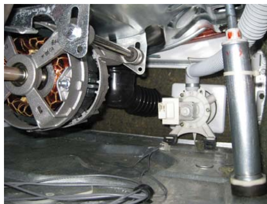
Figure 3.8 Drain pump and water outlet pipe
