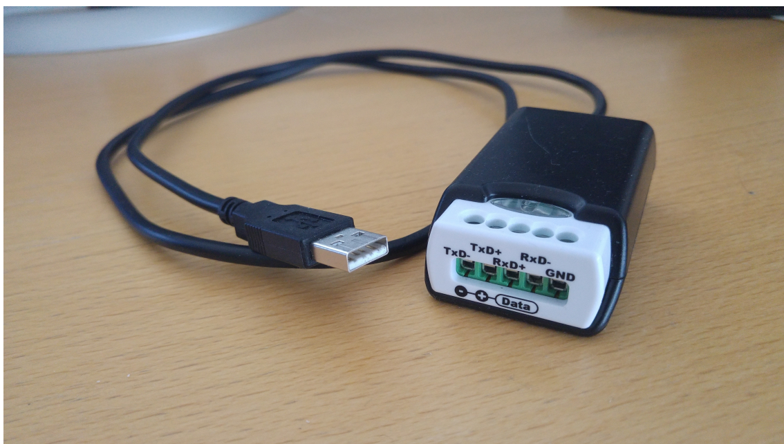
Figure 2.5: Titan USB-COMi-TB USB-to-Industrial Single RS-422/485 Adapter.
