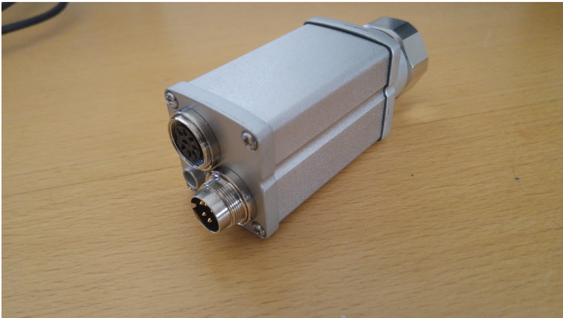
Figure 2.4: Comba RCU-003(VI) Remote Control Unit.
