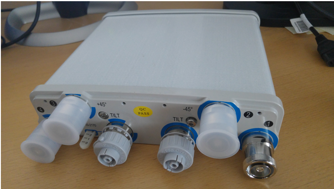
Figure 2.2: Comba ODU (Dual-band) Dummy antenna kit.
