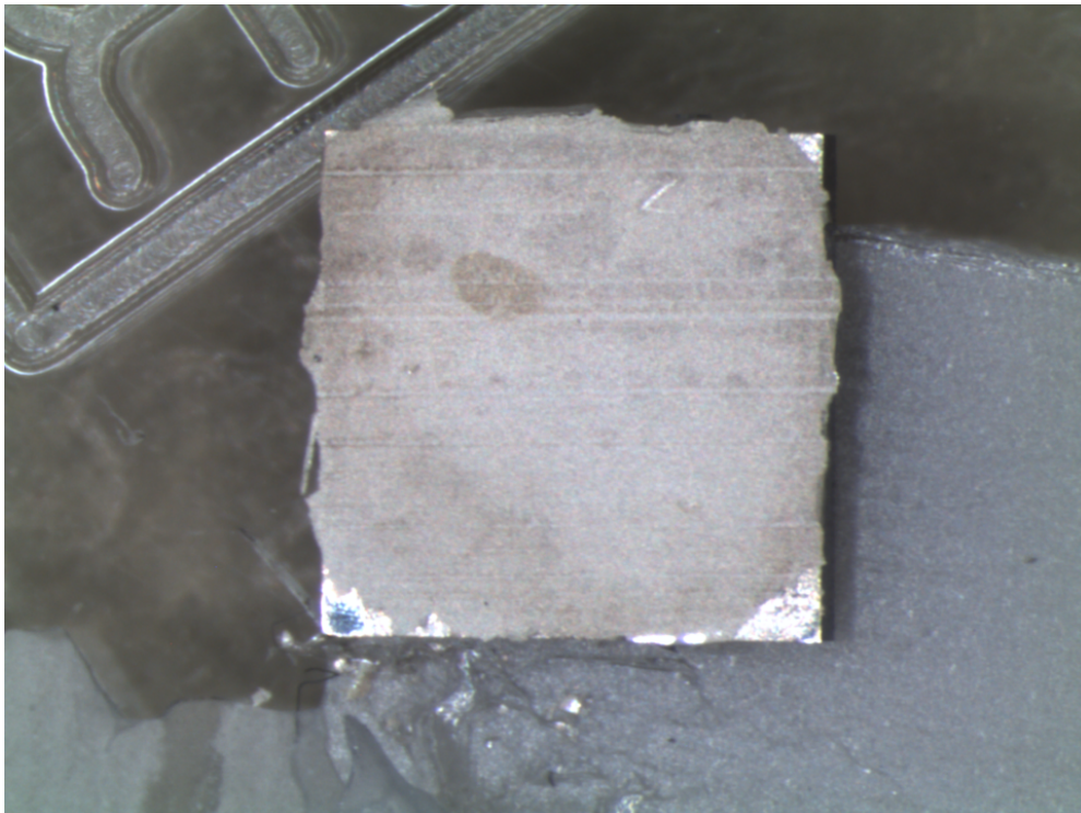
Figure 30 The lower surface of the released SiC chip.
