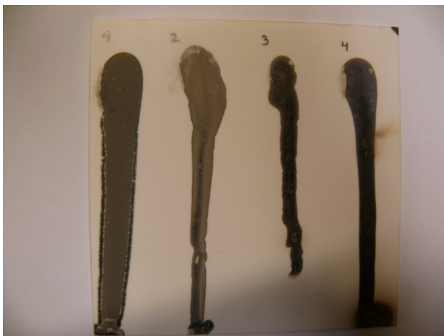
Figure 10 Result of experiment 1. Different concentrations of Tetraethyl Orthotitanate on \text{Al}_2\text{O}_3 after 1 hour in furnace.
