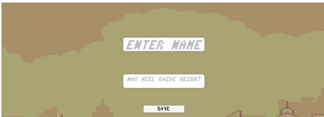
Figure 3.13: This is the menu for creating a new patient profile. You enter a name as well as a manually entered value for max heel raise height, which sets the game difficulty and was intended for future IMU implementation.
