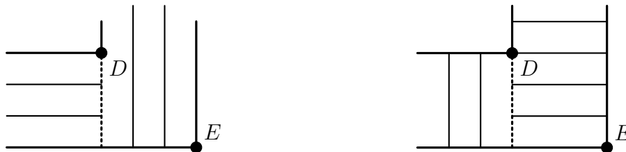
Figure 3.13: Two different sections of polygons that are identical except for the orientations of the strips. A switchline beginning in D can have E as its other endpoint in the left figure, but not the right. This is because in the left figure the strips opposite of E are perpendicular to the switchline, while the opposite is true for the right. Because of this, a switchline in the left figure can take on all monotone sequences between D and E while leaving the number of strips unchanged by extending and contracting strips, while some monotone sequences in the right figure can create new strips.
