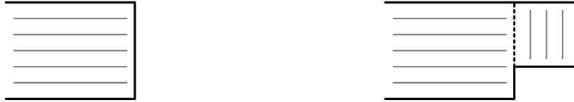
Figure 3.10: The two possible scenarios where one of the straight segments ends in a convex corner. In the first scenario, the switchline will overlap completely with the border and therefore disappear.
